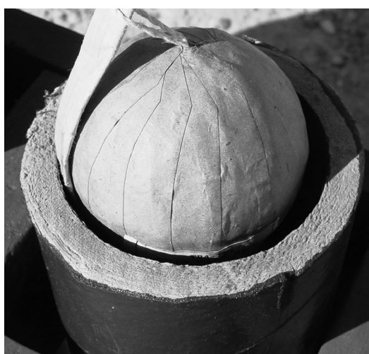
Leader fuse must be secured to the top of the shell. The shell below needs to be repaired.
