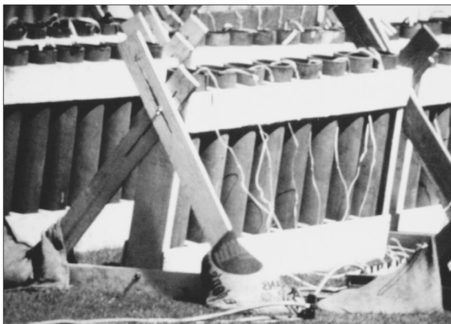
A wooden rack partially buried for stability.
