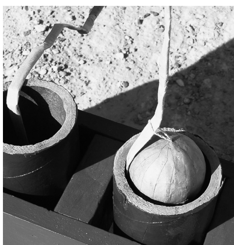
Leader fuse must be secured to the top of the shell. The shell below needs to be repaired.
