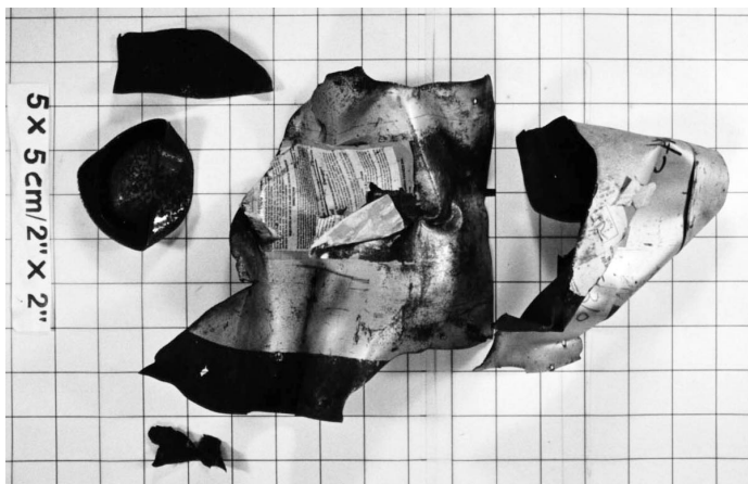
Result of salute exploding in a sheet steel mortar.
