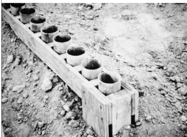
A wooden rack partially buried for stability.
